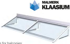
Our portfolio consists balcony roofs as well. Standard products for balconies up to 1300 mm depth are made of aluminium and welded to a uniform construction. Mounting brackets are easily accessible with power tools which makes installation easy. Balconies with depth more than 1300 mm, custom designed construction is produced.
